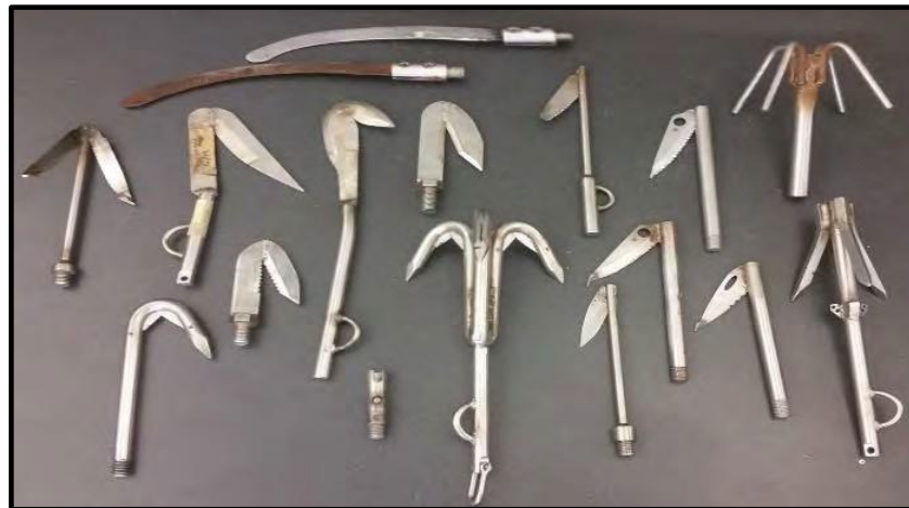
Figure 3: Cutting grapples that can be attached to ropes or poles and extended from the deck of a boat to cut entangling gear. Photo supplied by the Center for Coastal Studies ( https://coastalstudies.org/ ).
