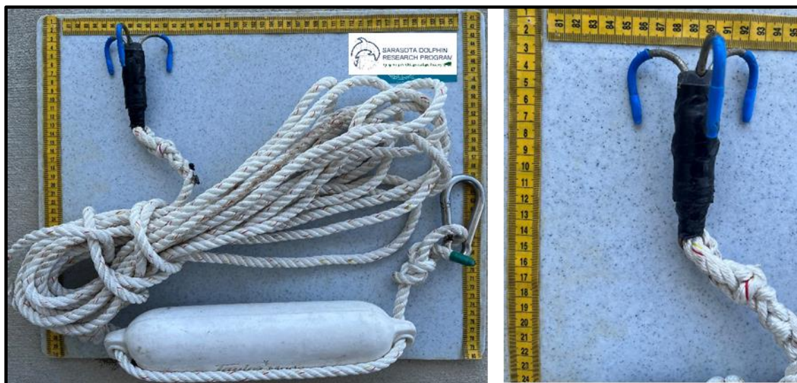
Figure 4: long-handled grapples with protected tips to avoid injury to the animal.
