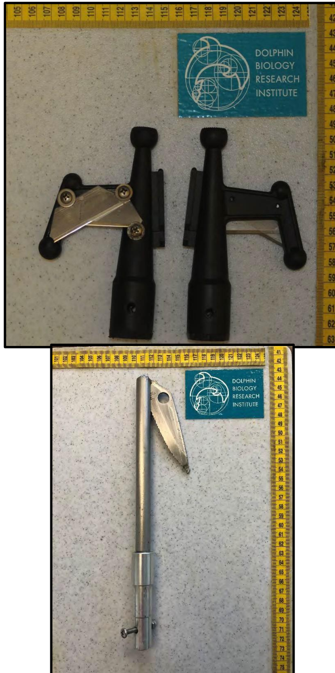
Figure 2: Specially designed cutting tools that can be fitted to the ends of long poles for use from the bow of a boat (Top photo courtesy of the Sarasota Dolphin Research Program, bottom tool designed by the Center for Coastal Studies).
