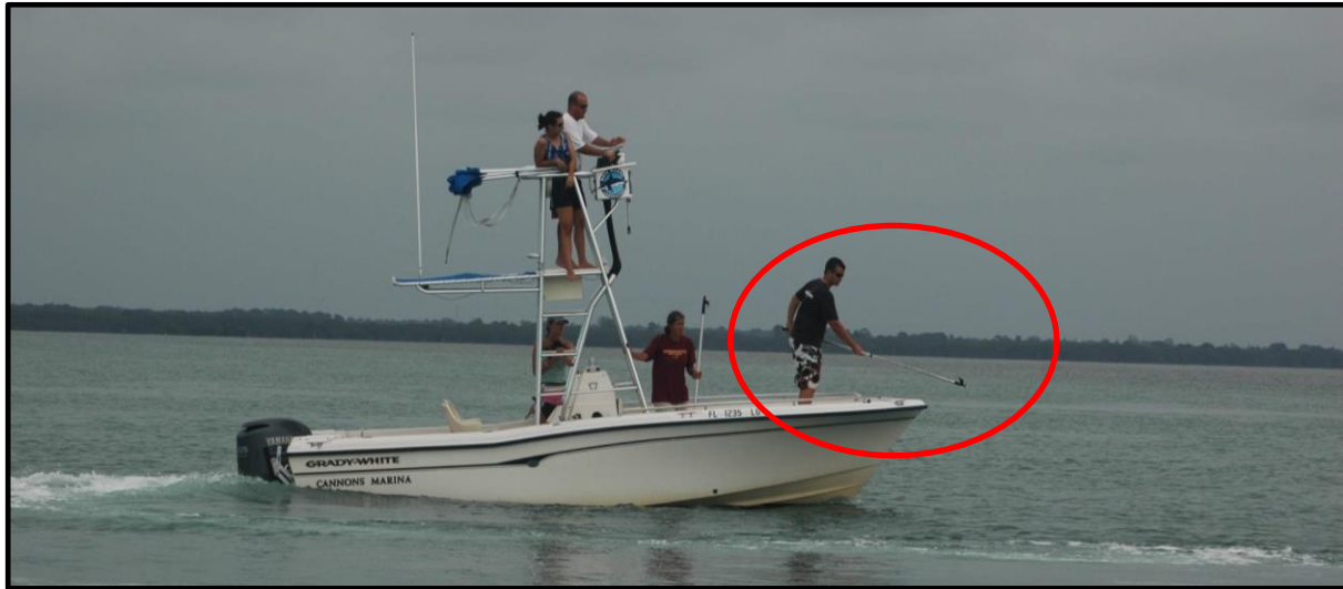
Figure 8: Vessel demonstrating the approach an animal for a remote disentanglement using a cutting tool mounted on a long handle. Note that the team members in this photo are not wearing life jackets/personal flotation devices, which is NOT recommended practice for actual interventions. ALL team members, especially those who will handle the tools and risk being pulled overboard if a tool is caught on the dolphin, should wear personal flotation devices and other protective equipment. Photo courtesy of the Sarasota Dolphin Research Program.
